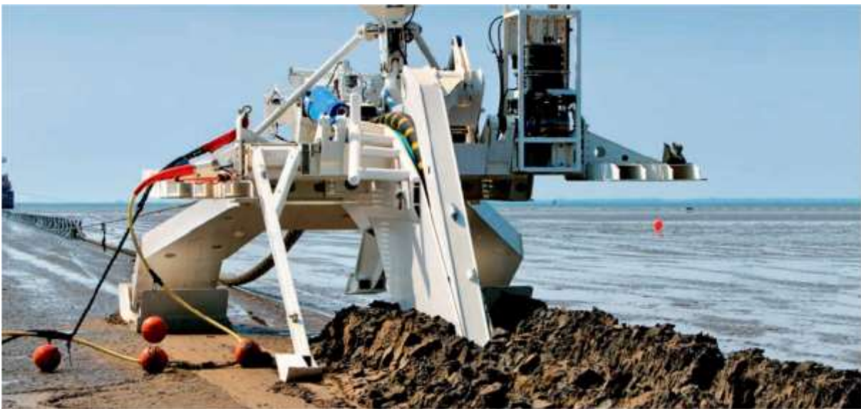
Figure 2.9. Example of a marine plow – Plough/Sea STALLION 4 DB model [Source: Boskalis: www.vbms.com ]
