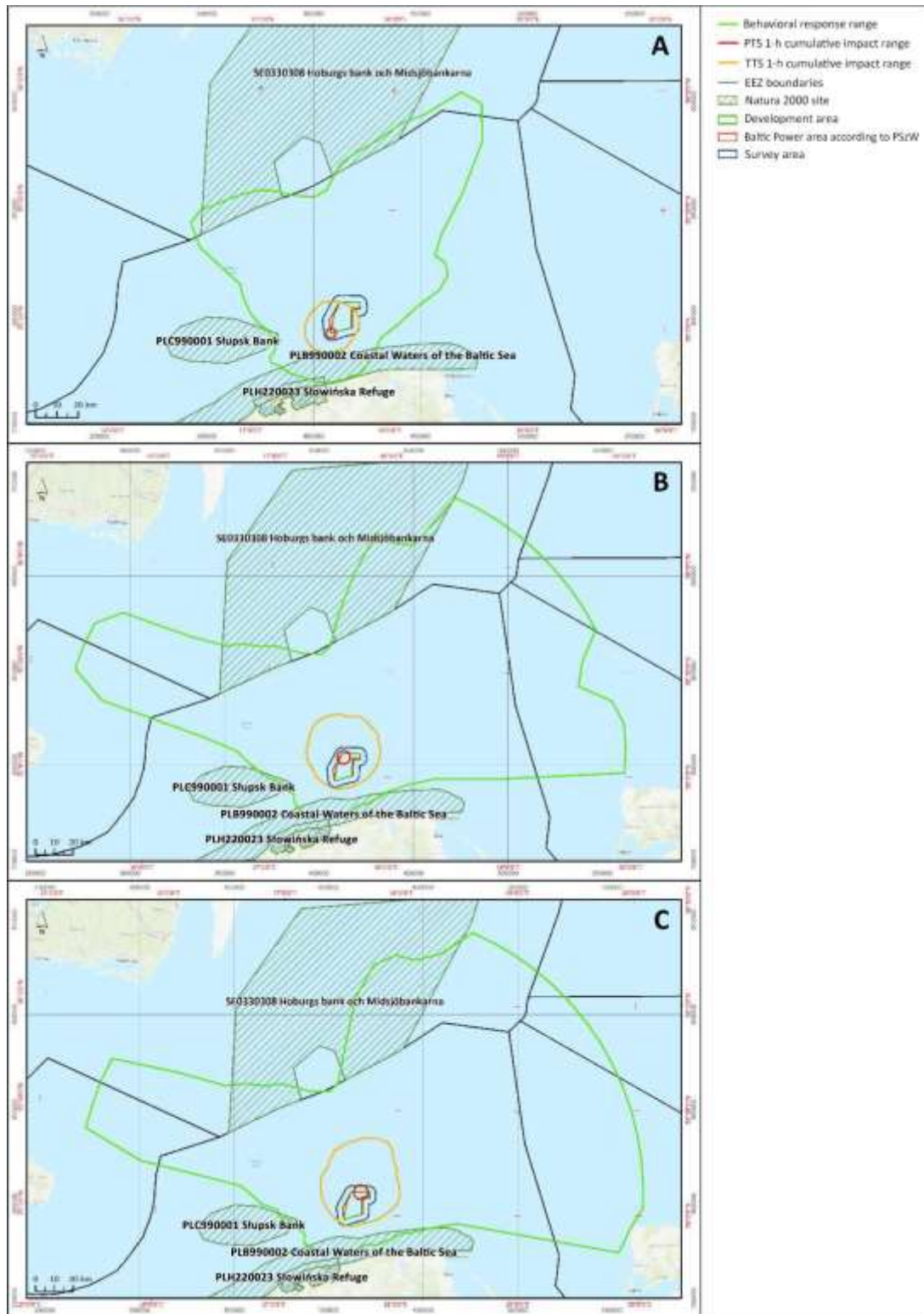
Figure 6.26. SEL unweighted noise propagation map for fish with a swim bladder from two close piling sources for turbines 1 (panel A), 40 (panel B) and 49 (panel C) in the Baltic Power OWF Area. The range of impacts was presented for fish with a swim bladder, including use of HSD [Source: data of Baltic Power Sp. z o.o.]
