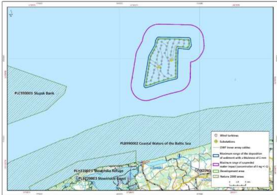
Figure 6.4. Range of impact of the increase in suspended matter content and the resulting sedimentation for the Baltic Power OWF [Source: own study]
