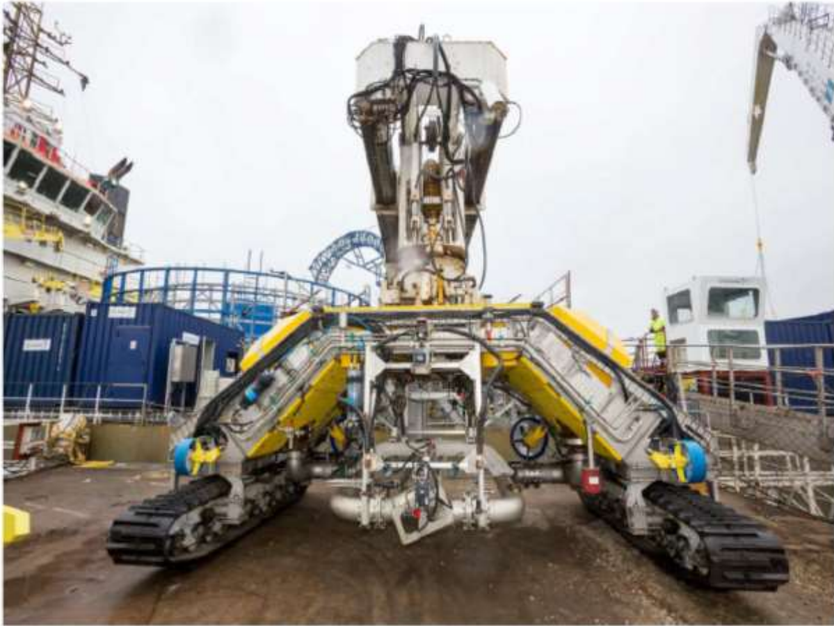
Figure 2.10. Example of ROV trencher – model ROV Trencher 107-1100 [Boskalis Source: www.vbms.com ]
