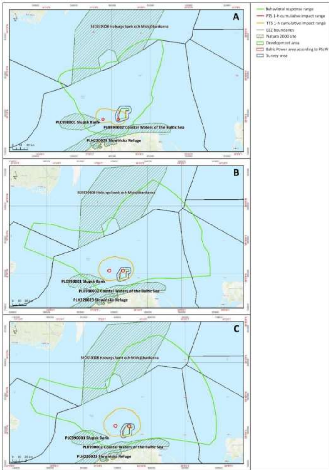
Figure 6.28. SEL unweighted noise propagation map for fish with a swim bladder from two piling sources located 20 km (average distance) apart for turbines 1 (panel A), 40 (panel B) and 49 (panel C) in the Baltic Power OWF Area. The range of impacts was presented for fish with a swim bladder, including use of HSD [Source: data of Baltic Power Sp. z o.o.]
